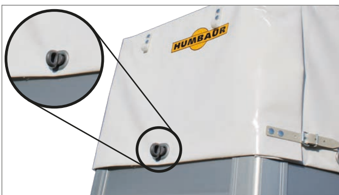
Front side of tarpaulin section, staple / buckles secured
