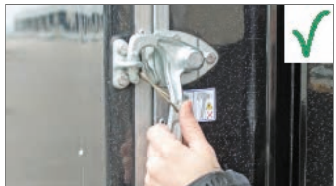
Securing the revolving door at the top
