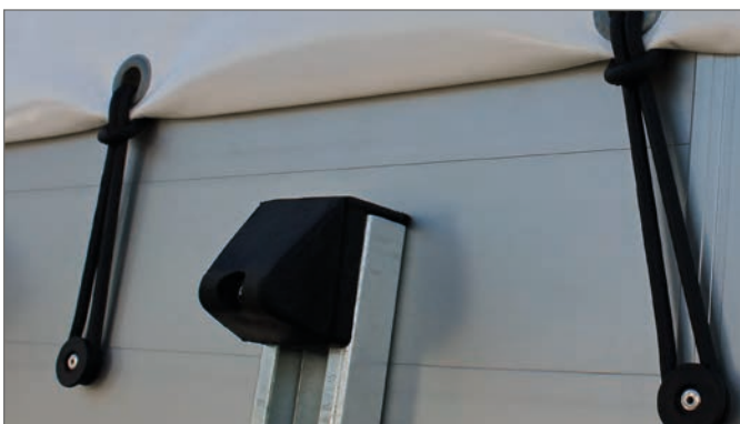
Tarpaulin section rear side, elastic cord fastener secured
