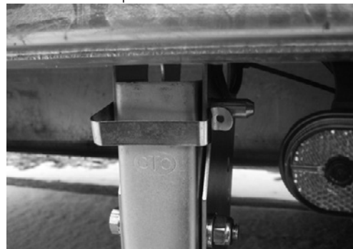
Setting the underrun protection with a bolt
