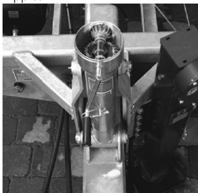
Lubricating the drawbar
