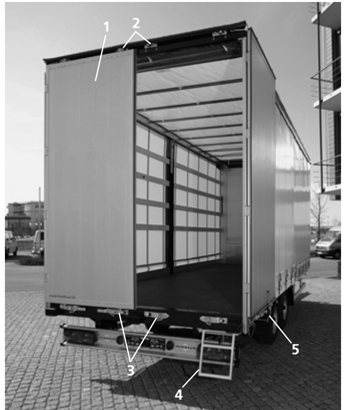
Rear view of the HT with curtainsider structure
