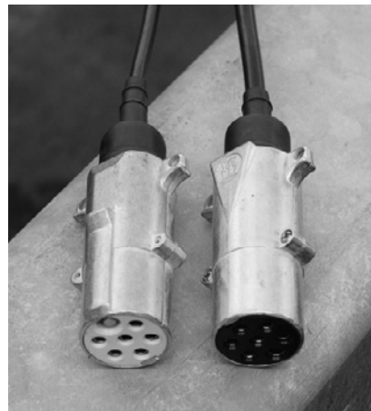
7-pin normal plug and 7-pin additional plug
