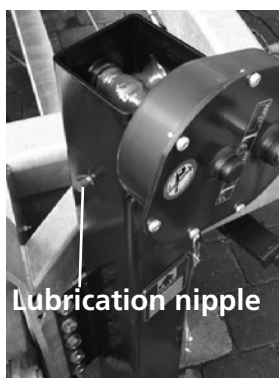
Lubricating the supporting base
