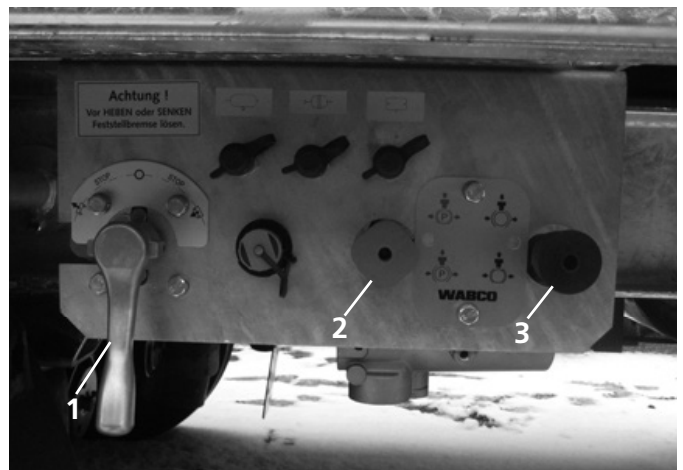
Brake control panel for trailers with pneumatic suspension
