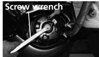
Spring brake with screw wrench
