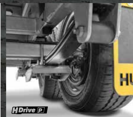
PARABOLIC SUSPENSION Low suspension travel, maximum comfort
