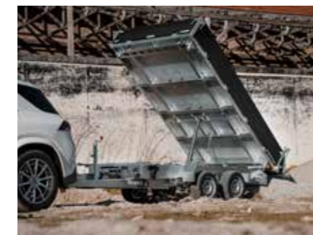
The HTK can be tilted backwards and sideways in a few simple steps.
