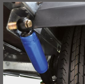
Wheel shock absorbers (mounted), with 100 km/h confirmation; wheel shock absorbers (loose) without 100 km/h confirmation
