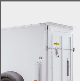
Ramp wall instead of rear door
