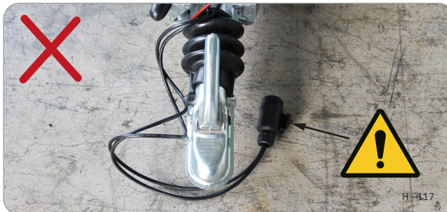
Cable plug stowed incorrectly
