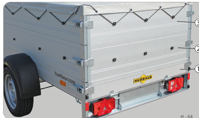
Example: Double side wall extension (Multi)
