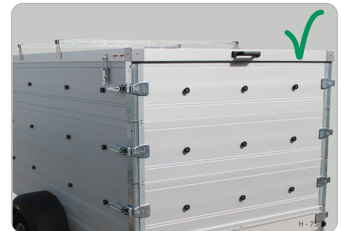
Aluminium cover closed / locked (driving position)
