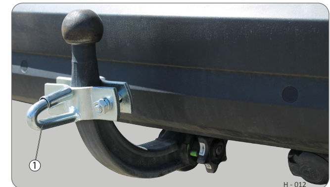
Example: Coupling with clamping device
