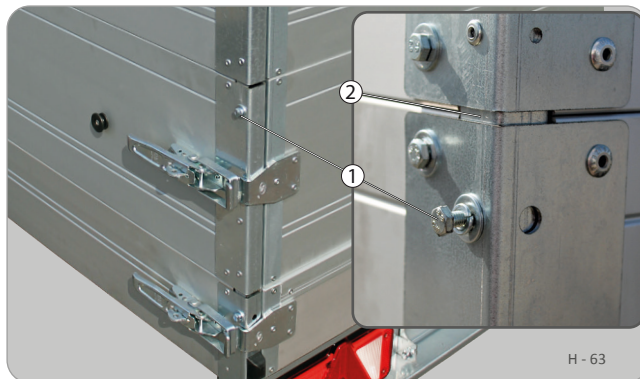
Side wall extension secured
