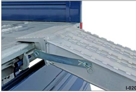
**Fig. 13** Patented locking mechanism
