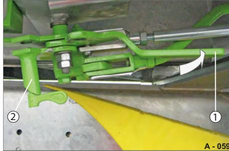
**Fig. 56** Closing central locking system
