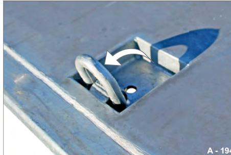
**Fig. 205** Lashing ring folded out
