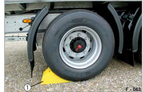
**Fig. 88** Wheel chocks in place
