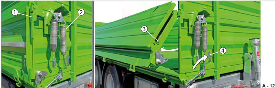
Fig. 131 Base platform gate with folded down platform gate attachment swinging
