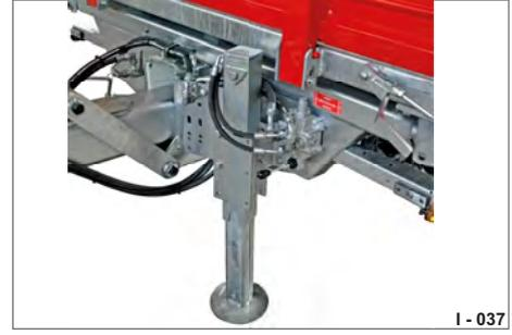
**Fig. 27 Hydraulic support equipment**
