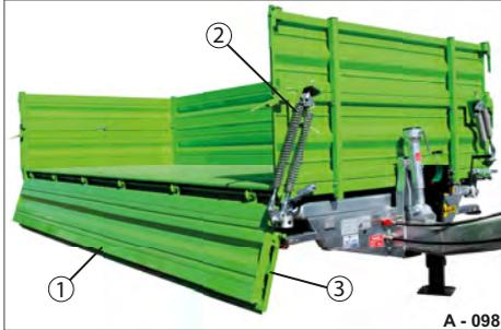
**Fig. 100** Steel platform gate attachments
