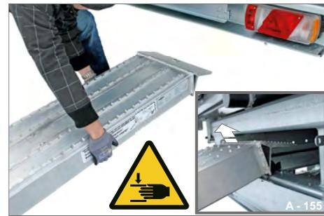
Fig. 165 Lifting out ramp planks
