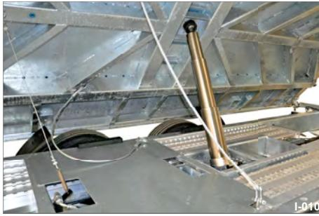
**Fig. 12** Loading bridge tilted to the side
