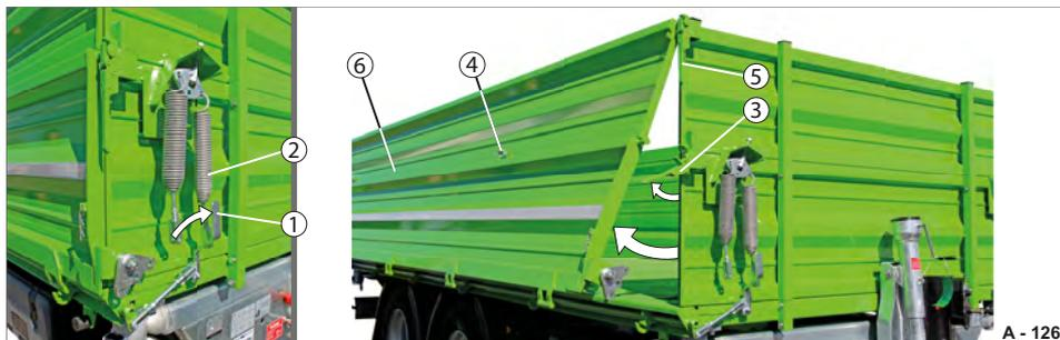
Fig. 132 Base platform gate with folded down platform gate attachment swinging
