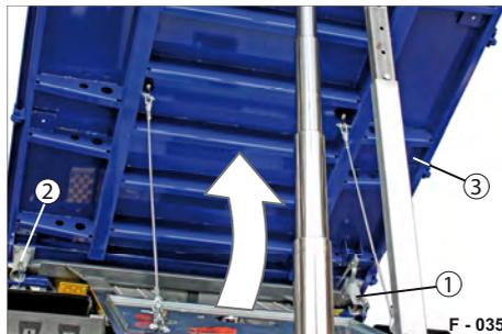
**Fig. 58** Tilting loading platform backwards
