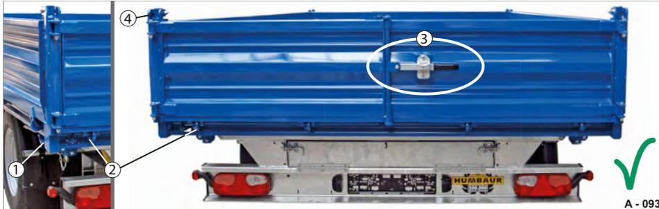
Fig. 77 Central locking system for pendulum mode:
