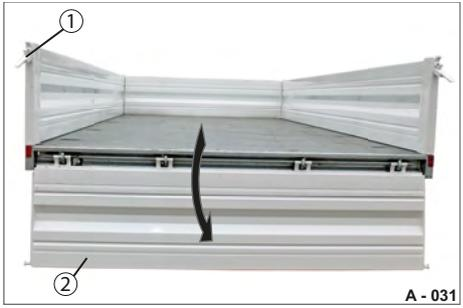
**Fig. 39** Rear platform gate, folded down
