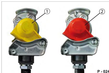
**Fig. 4** Brake/supply line disconnected
