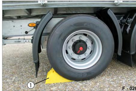
**Fig. 17** Trailer secured
