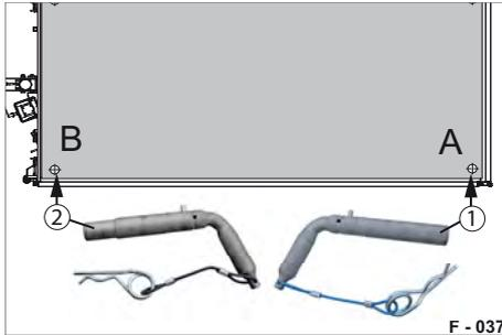
**Fig. 60** Socket pins inserted in left direction of travel
