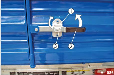
**Fig. 71** Locking lever secured
