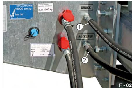
**Fig. 46** Hydraulics as 2-circuit system
