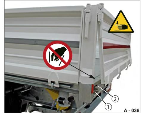
Fig. 44 Central locking system unlocked
