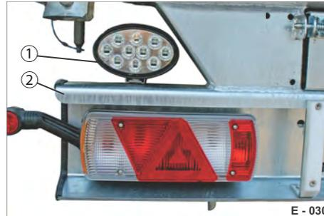
**Fig. 25** Working lights at rear;
