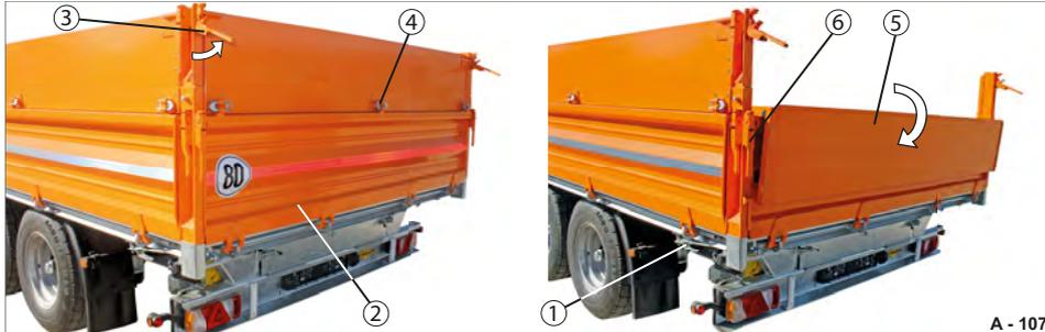
Fig. 114 Rear platform gate attachment, folded down
