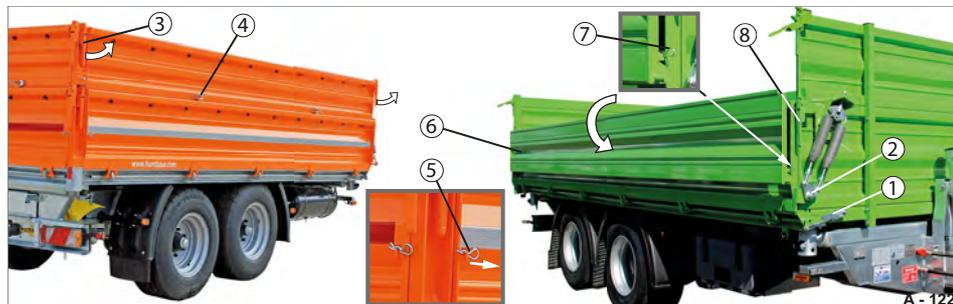
Fig. 128 Platform gate attachment folded to the side
