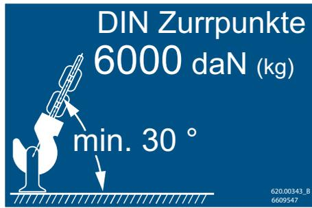
**Fig. 199** Sign for lashing ring
