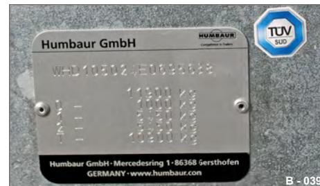
Fig. 18 Nameplate/weight specifications
