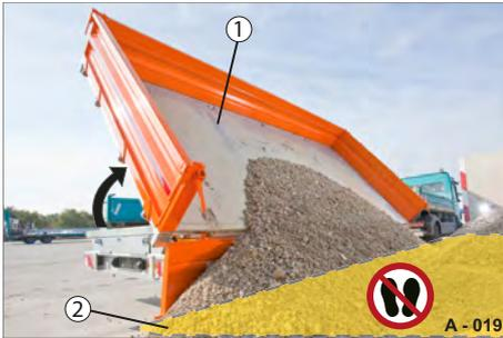
**Fig. 21** Loading platform, tilted to the side
