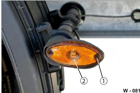
**Fig. 79** Side marking light "LED"
