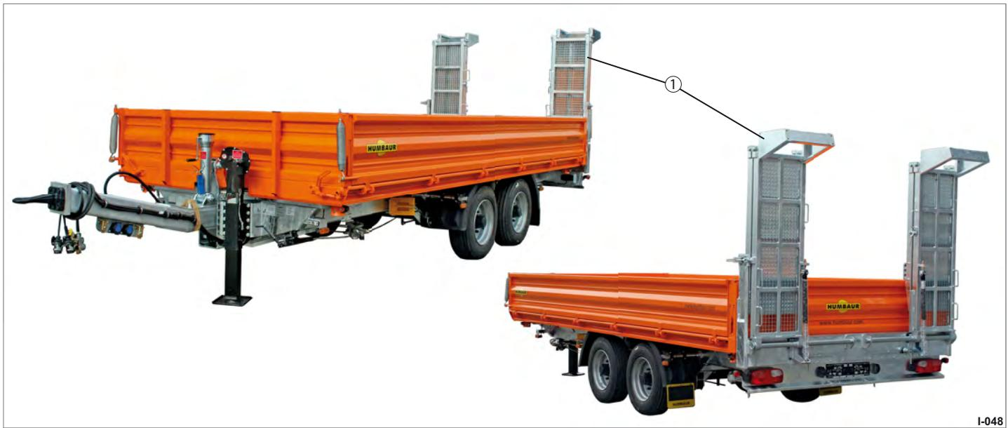
**Fig. 8** HTK with stationary ramps
