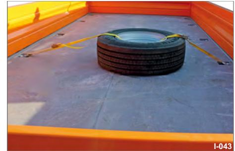
Fig. 32 Loose spare wheel on the loading platform
