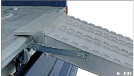
**Fig. 170** Ramp planks with securing hooks
