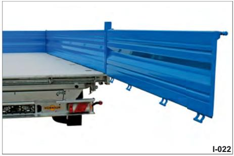
Fig. 36 Rear platform gate as swinging door
