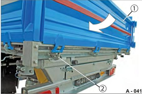
**Fig. 55** Rear platform gate closed
