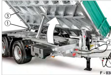
**Fig. 61** Loading platform tilted to the side
