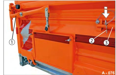
**Fig. 98** Operating lever, secured
