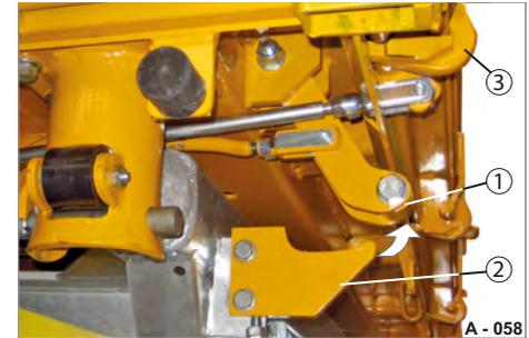
**Fig. 54** Rear platform gate unlocked
