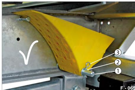
**Fig. 90** Wheel chock, secured
