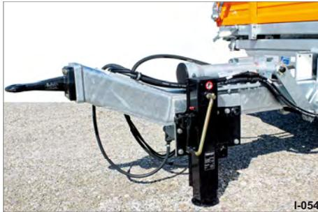
Fig. 28 Swivelable support equipment for through-load option
