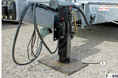
**Fig. 68** Support foot stabilised
