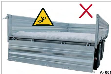
Fig. 1 Loading platform with snow/ice on top
