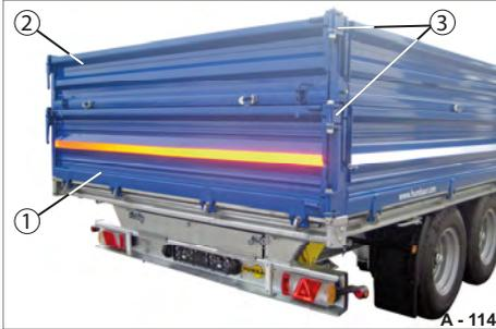
**Fig. 101** Swinging gate function
