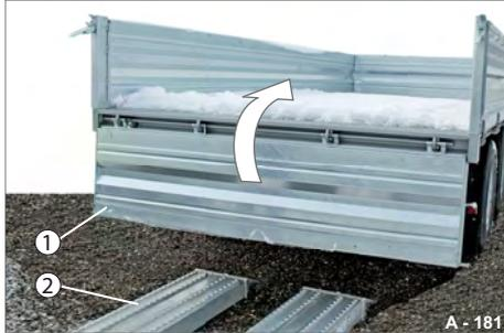
**Fig. 192** Closing rear platform gate
