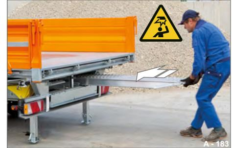
**Fig. 194** Sliding in ramp planks
