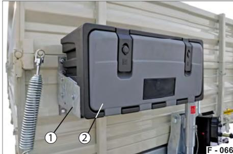
Fig. 91 Toolbox on the front wall
