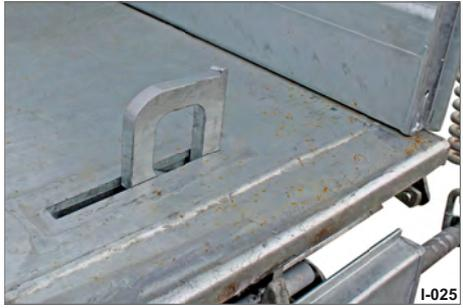
Fig. 37 Blade lashing ring, retractable
