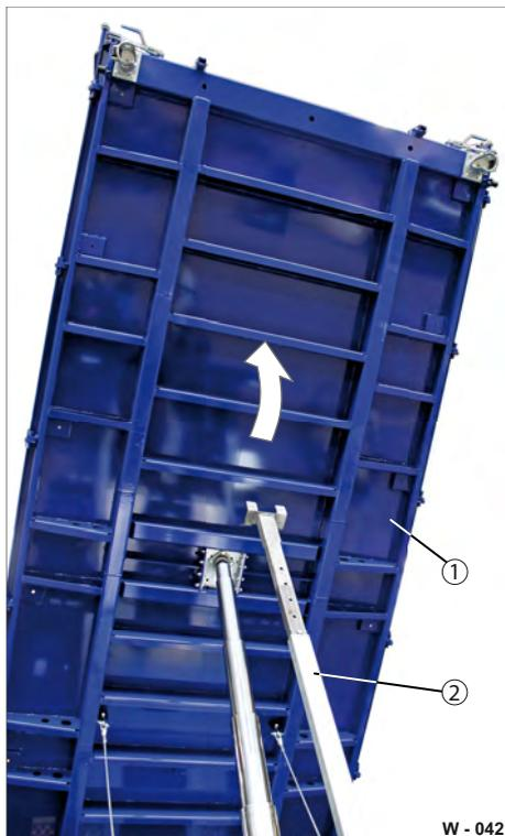
**Fig. 42** Folding down service support
