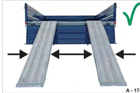
Fig. 185 Positioning ramp planks
