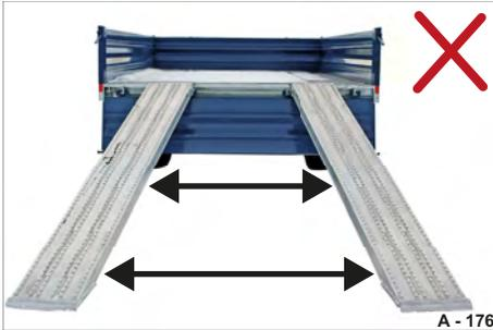
Fig. 184 Ramp planks positioned at an angle
