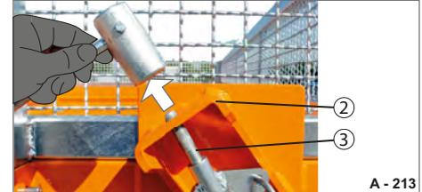
**Fig. 125** Releasing lifting springs
