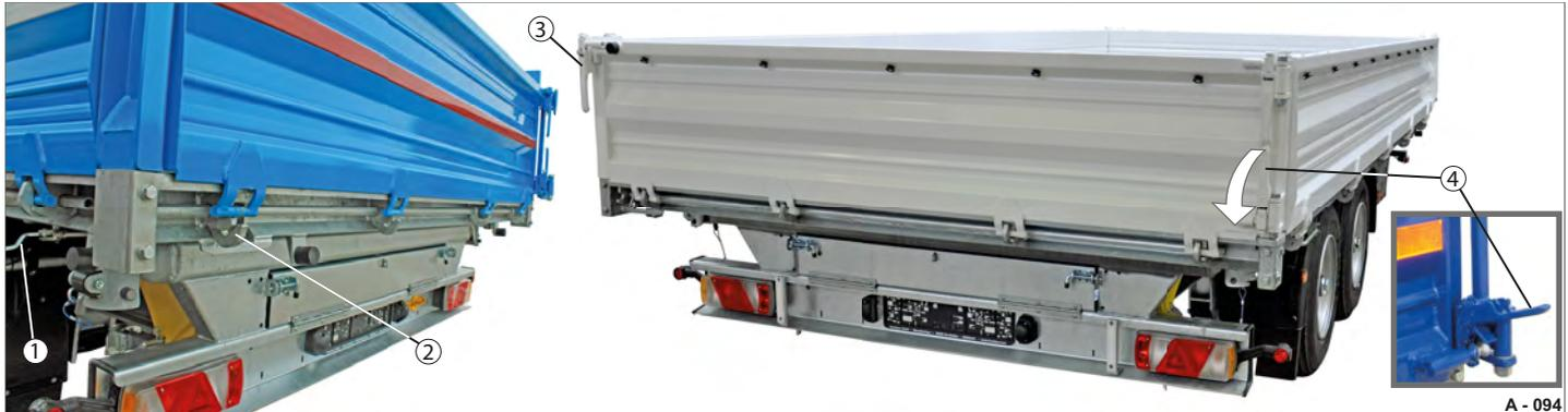
Fig. 68 Swinging gate in pendulum mode
