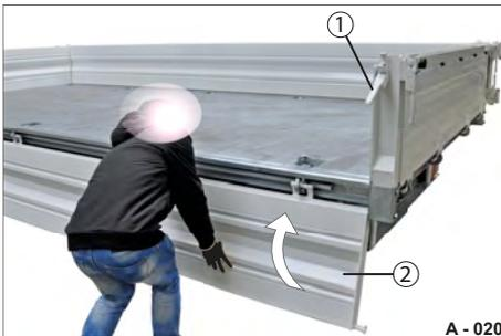
**Fig. 22** Fold up platform gate
