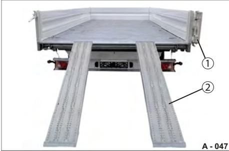
**Fig. 65** Ramp planks positioned
