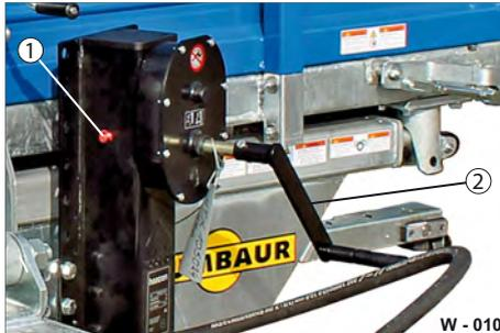
**Fig. 10** Gear-supported jack on chassis
