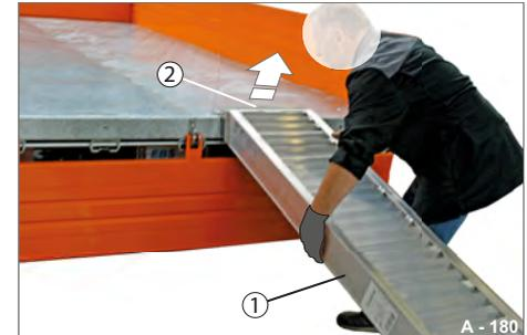
**Fig. 191** Setting ramp planks down
