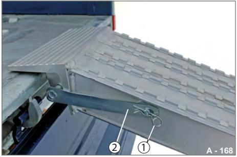
**Fig. 179** Securing the locking lever
