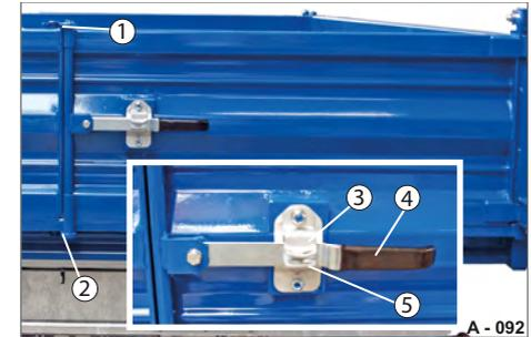
**Fig. 76** Swinging gate secured
