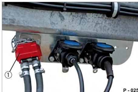
**Fig. 5** Duo-Matic quick-release coupling system
