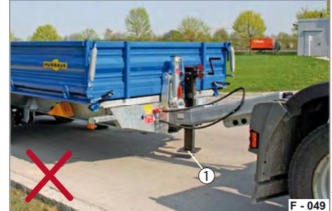
**Fig. 69** Driving with lowered support foot
