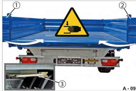
**Fig. 75** Closing swinging gate
