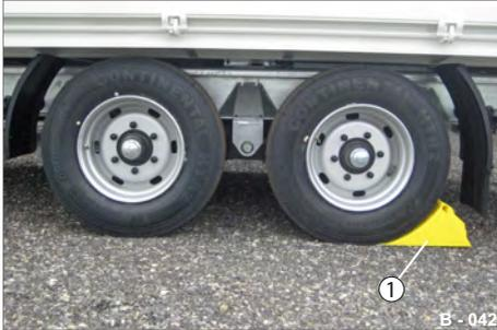
**Fig. 48** Wheel chocks positioned
