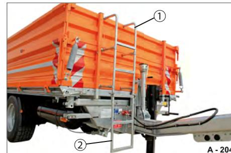
**Fig. 221** Access ladder folded out
