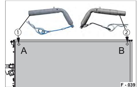
**Fig. 62** Socket pins inserted in right direction of travel
