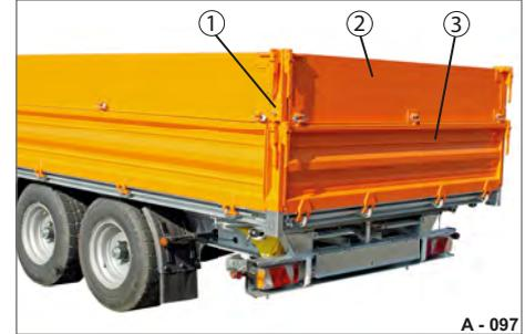
**Fig. 103** Aluminium platform gate attachment
