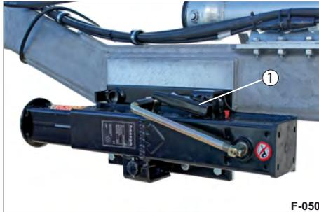
**Fig. 75** Swivel support/drive position
