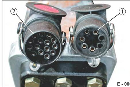
**Fig. 2** Plug-in connections, standard 24 V
