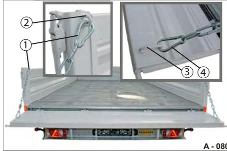
**Fig. 81** Rear platform gate secured
