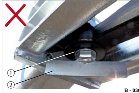
**Fig. 39** Incorrectly secured - view, bottom
