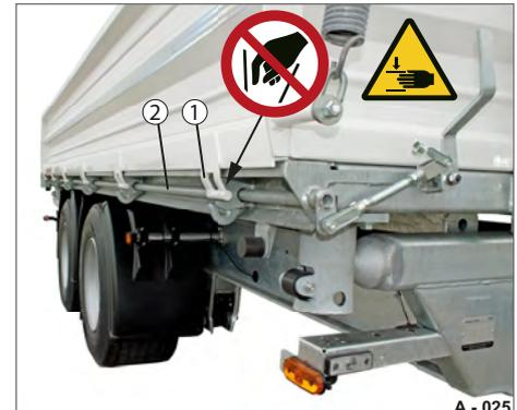
**Fig. 27** Central locking system unlocked
