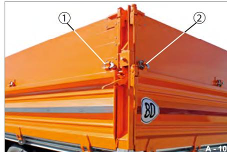
**Fig. 109** Hinges, secured on all sides
