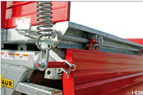
Fig. 41 Guard lock of the side platform gates
