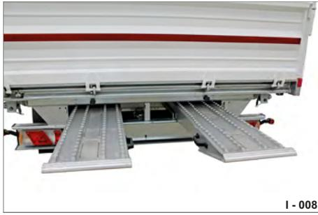
**Fig. 10** Ramp plank bays in chassis
