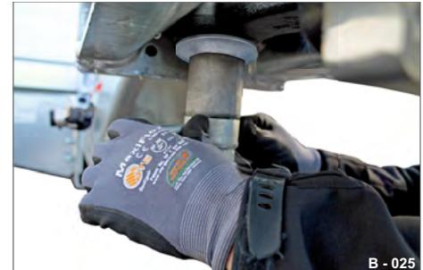
**Fig. 34** Towing eye D50 secured
