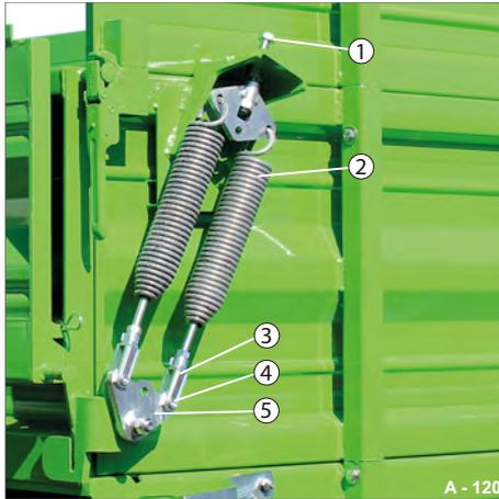
**Fig. 121** Lifting springs, suspended
