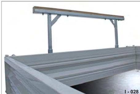
**Fig. 17** Support frame on front platform gate, e.g. for wheel loader/excavator shovel
