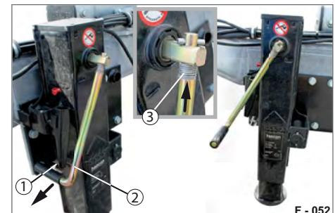
**Fig. 77** Swivel support - support position
