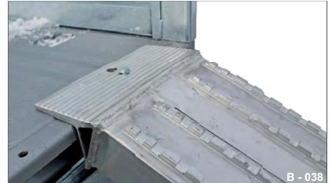
**Fig. 172** Ramp planks with retaining pin
