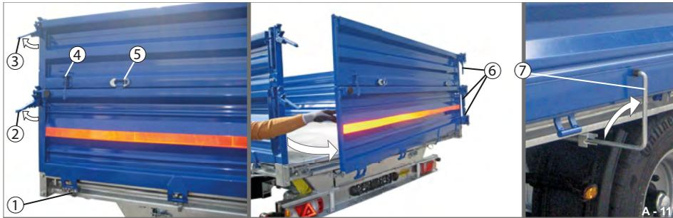
**Fig. 118** Opening rear platform gate with platform gate attachment as swinging gate
