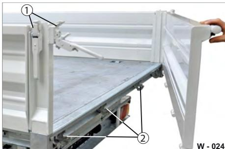
**Fig. 24** Lubrication points
