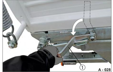
**Fig. 30** Lock central locking system
