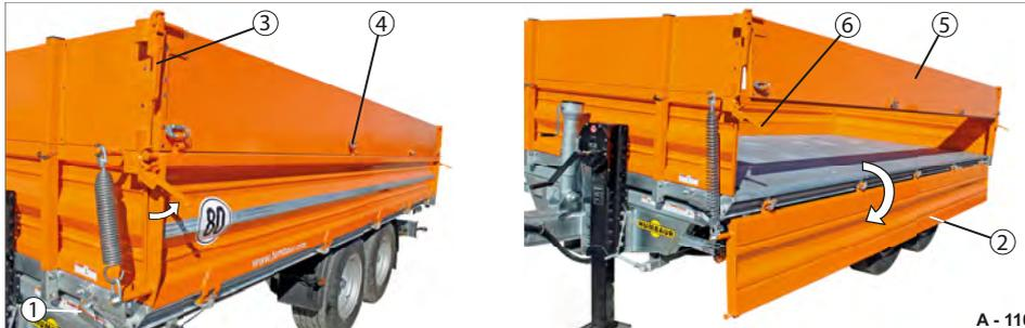
Fig. 113 Base platform gate folded down/platform gate attachment swinging
