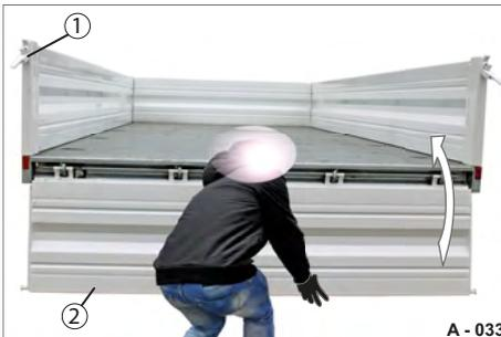
**Fig. 41** Fold up rear platform gate
