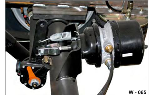
**Fig. 65** Releasing spring tension
