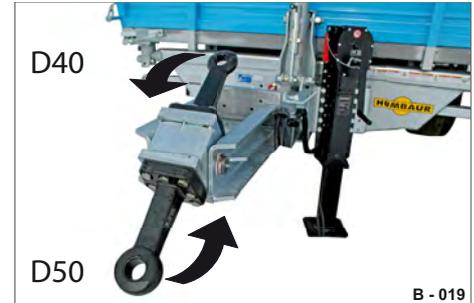
**Fig. 28** Turning the towing eye
