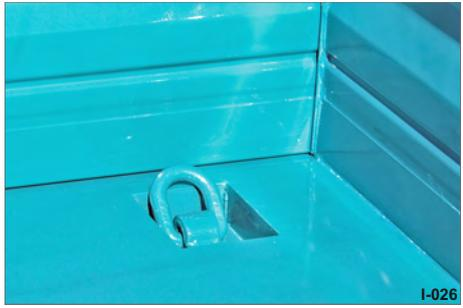
Fig. 34 Lashing ring, can retract in pocket
