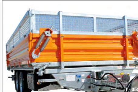
**Fig. 18** With dual lifting springs
