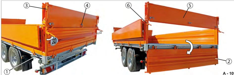
Fig. 115 Rear platform gate/platform gate attachment swinging
