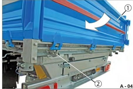
**Fig. 49** Rear platform gate closed
