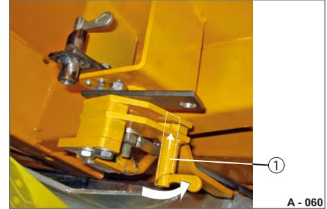
**Fig. 57** Central locking system secured
