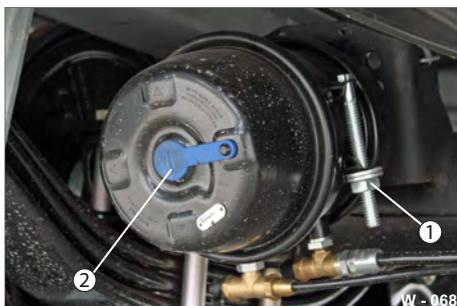
**Fig. 66** Spring-loaded diaphragm cylinder
