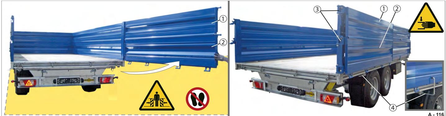
Fig. 117 Rear platform gate as swinging gate
