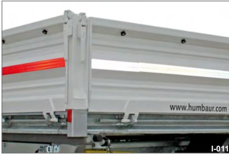
**Fig. 15** Round buttons on platform gates
