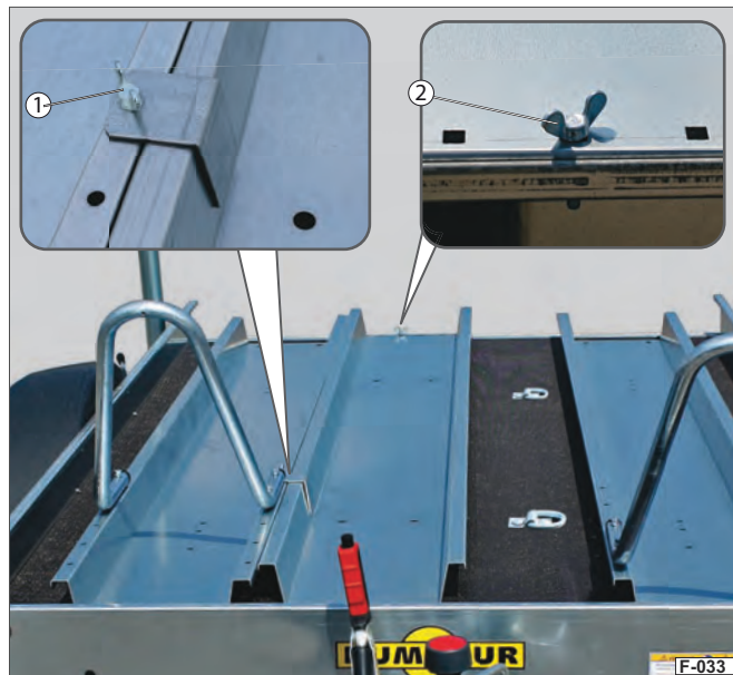
Fig. 26 Loading ramp secured (driving position)
