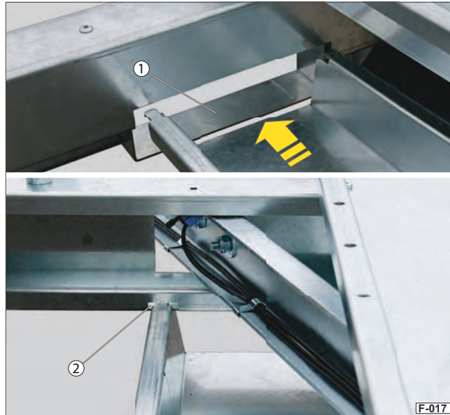
Fig. 17 Inserting the loading ramp
