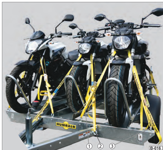
Fig. 16 Motorcycles secured at the front
