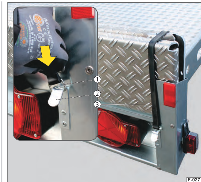
Fig. 35 Loading ramps secured (driving position)
