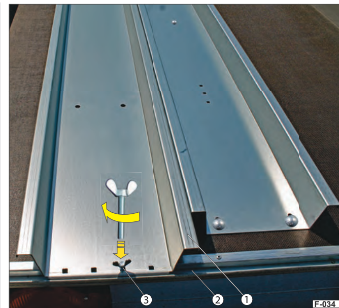
Fig. 24 Loading ramps positioned
