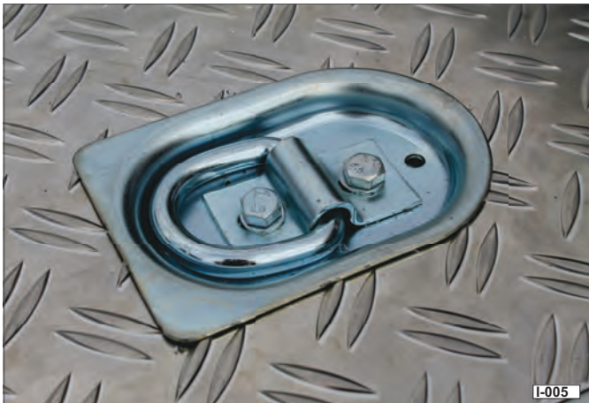
Fig. 6 recessed in the floor (hollow pocket)
