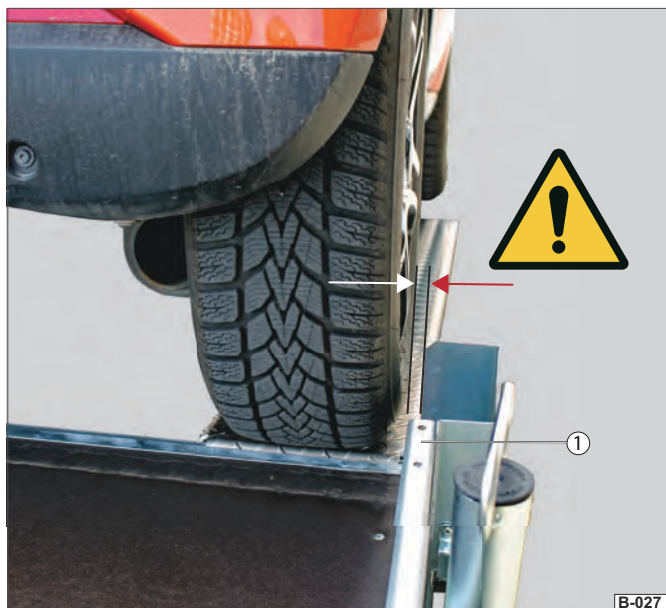
Fig. 26 Distance: Tyres - steel skirt
