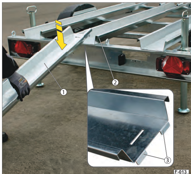
Fig. 13 Positioning the loading ramp
