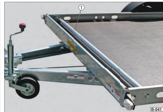
Fig. 47 Wheel stop, in position
