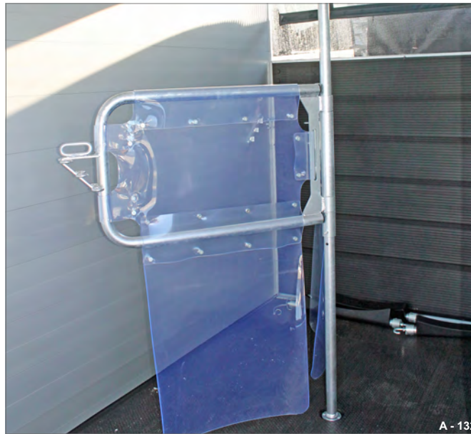
Fig. 132 Turned position of the central partition wall (Notos)
