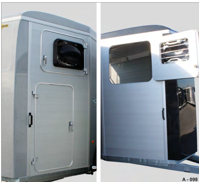
Fig. 98 Ventilation window closed / open
