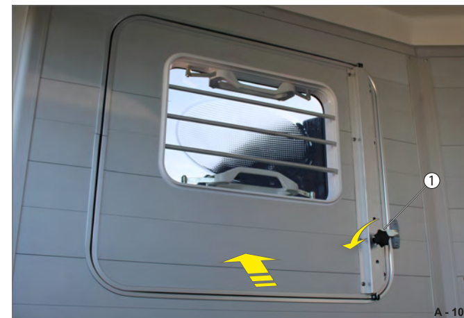
Fig. 101 Opening the ventilation window from the inside
