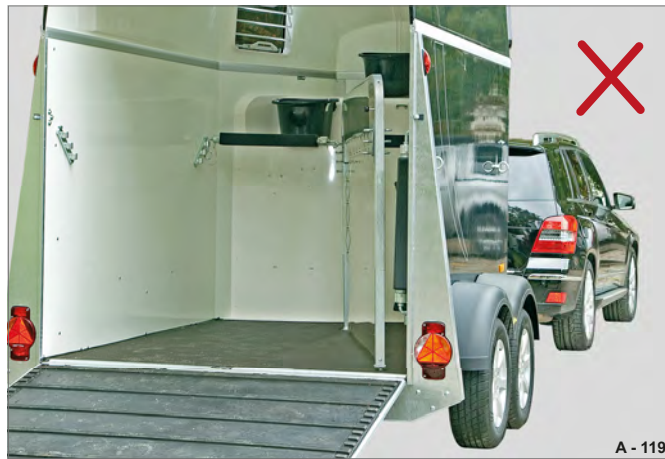
Fig. 119 Central partition wall not secured
