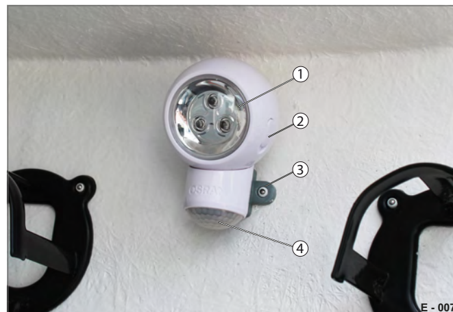
Fig. 7 LED light with movement detector
