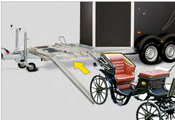
Fig. 11 Driving on the loading ramps
