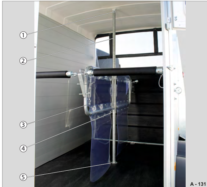
Fig. 131 Central partition walls (Notos)
