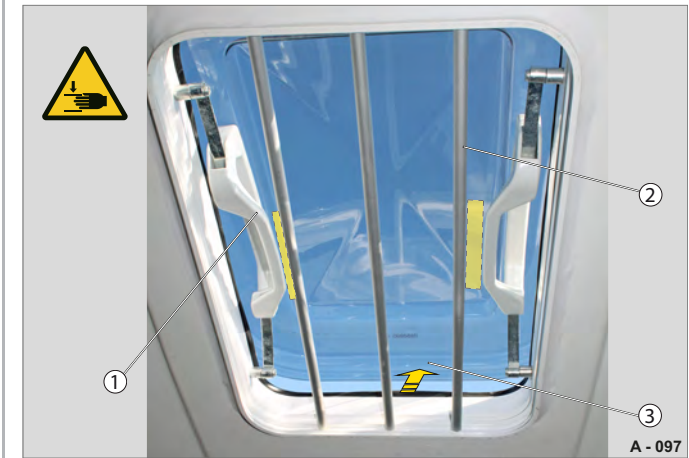
Fig. 97 Skylight opened (in driving direction)
