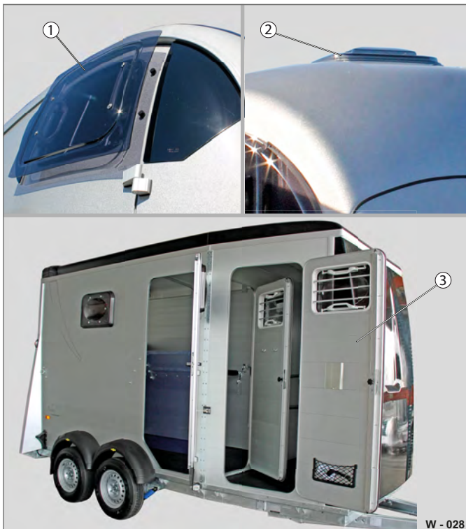
Fig. 28 Ventilating the trailer / drying it out
